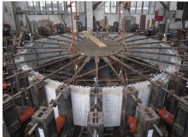
**Fig. 1:** Geometry and loading configuration of the tunnel
