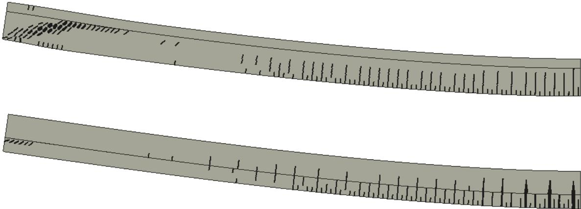
Fig. 8. Typical shear (top) and bending (bottom) failure in finite element model
