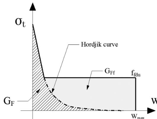
Fig. 7. Used tensile function for numerical calculation
