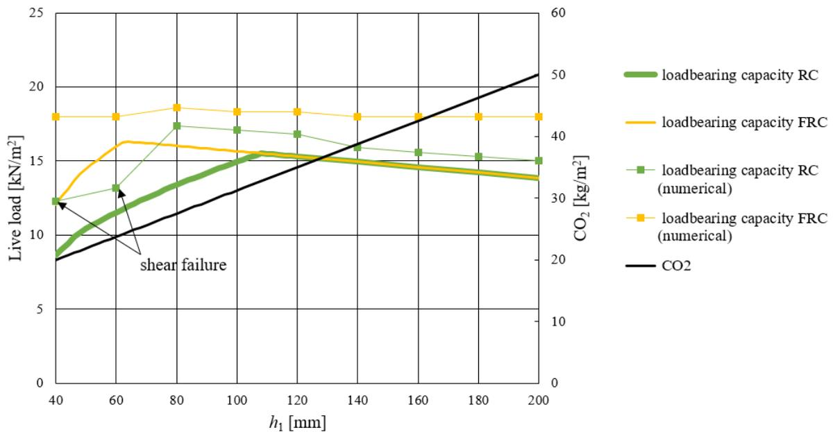
Fig. 9. Results of numerical model and CO<sub>2</sub> emission
