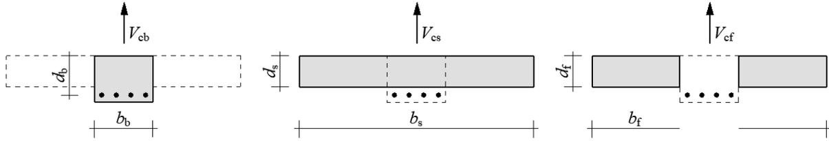
Fig. 3. Definition of shear capacity
