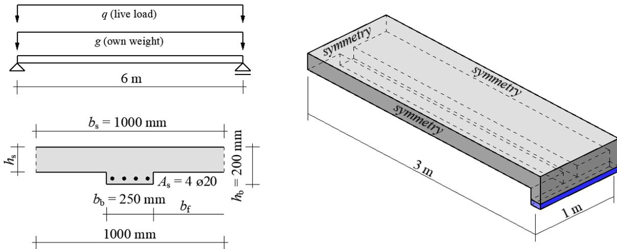
Fig. 2. Geometry of the structure
