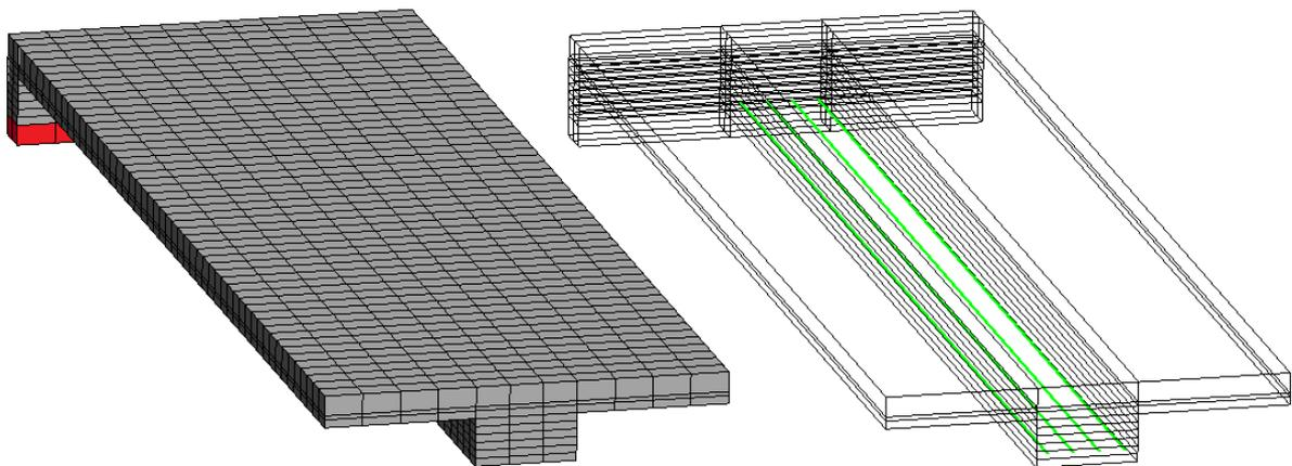
Fig. 5. Slab calculation with ATENA, red: support, grey: PC/FRC, green: steel bars
