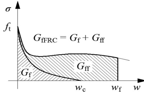
Fig. 6. Fracture energy of the FRC [26]
